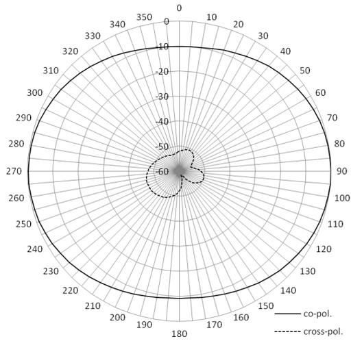
Fig. 6 The calculated radiation pattern,  $H$ -plane ( $xz$ ), 993 MHz
