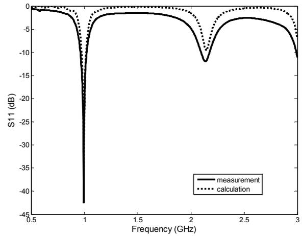
Fig. 4 Measured and calculated results for the return loss, diodes in the off state
