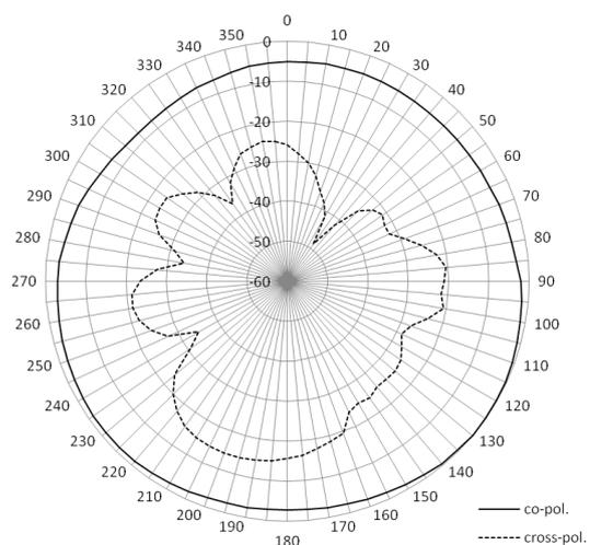
Fig. 11 The measured radiation pattern,  $H$ -plane ( $xz$ ), 1940 MHz
