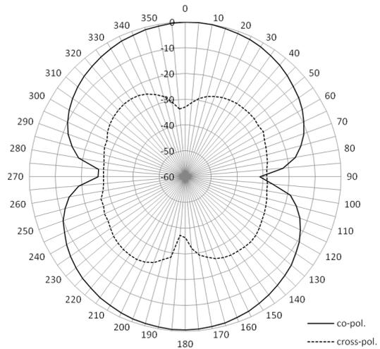
Fig. 9 The measured radiation pattern,  $E$ -plane ( $xy$ ), 993 MHz
