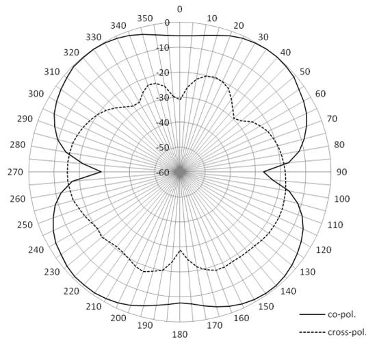
Fig. 13 The measured radiation pattern,  $E$ -plane ( $xy$ ), 1940 MHz
