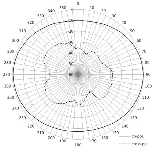
Fig. 7 The measured radiation pattern,  $H$ -plane ( $xz$ ), 993 MHz
