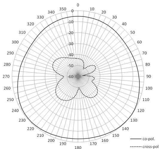
Fig. 10 The calculated radiation pattern,  $H$ -plane ( $xz$ ), 1940 MHz
