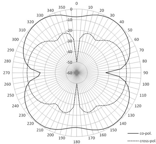
Fig. 12 The calculated radiation pattern,  $E$ -plane ( $xy$ ), 1940 MHz
