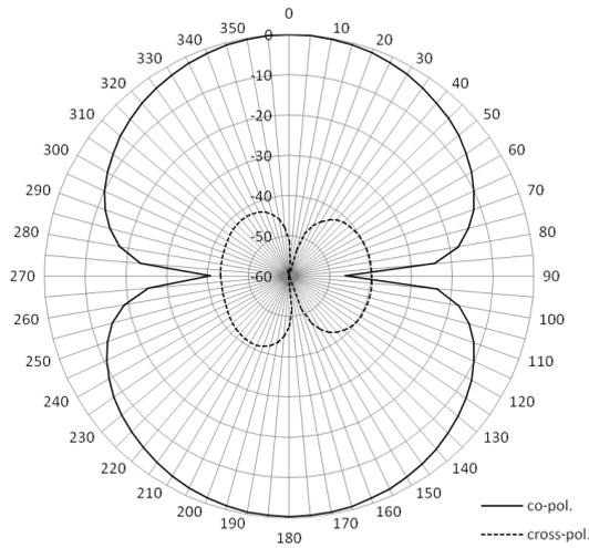
Fig. 8 The calculated radiation pattern,  $E$ -plane ( $xy$ ), 993 MHz
