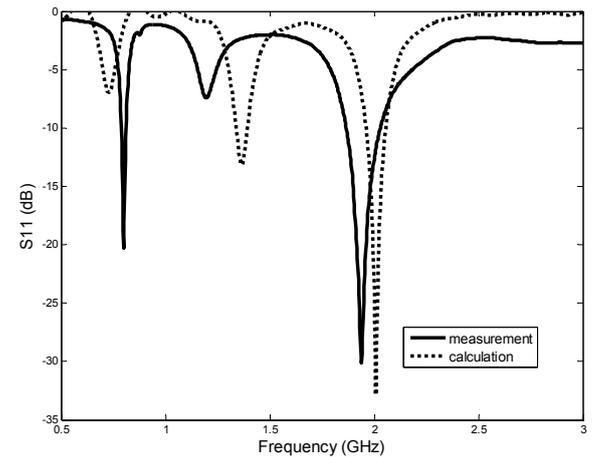
Fig. 5 Measured and calculated results for the return loss, diodes in the on state
